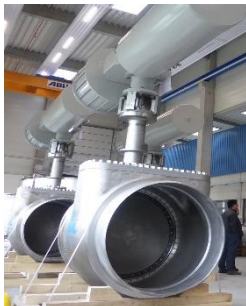
REACTOR SWITCHING VALVES
